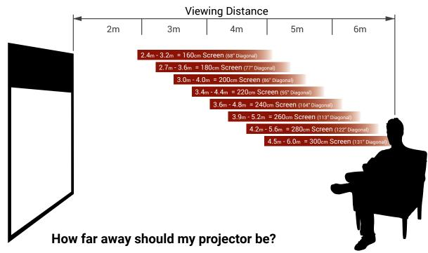
All projectors have different throw ratios. This simply determins the minimum & maximum distance from the projector to the screen.
